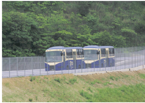
Automatic drive system operating in the bus fleet at the Awaji Farm Park on Awaji Island. This is part of Toyota Motor Company's IMTS (Intelligent Multimode Transport System) development.
