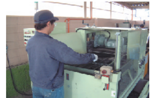
Integrated iron and glass grinding/ separating equipment
