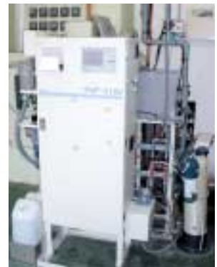
Fully automatic continual measuring apparatus for nitrogen and phosphorus
