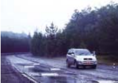
Durability test on a looped rough road track
