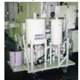
Waste oil filtration system
